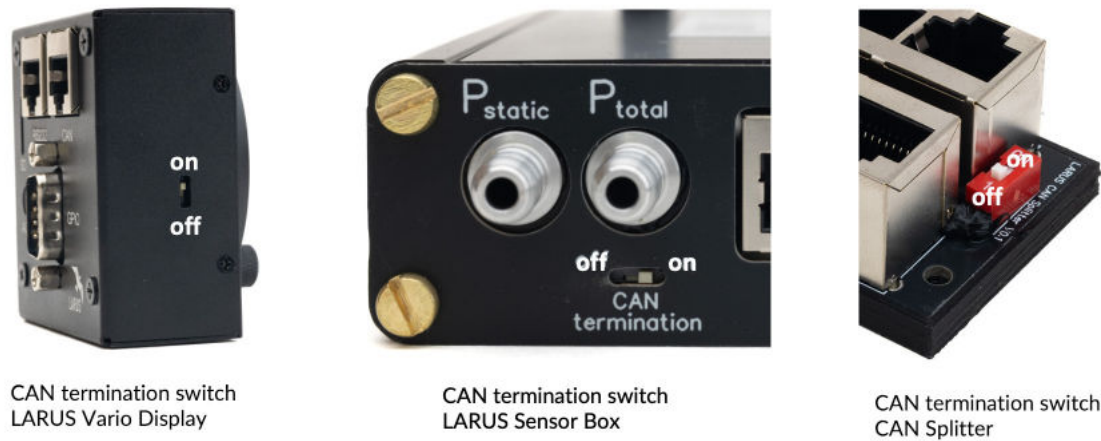
Figure 6: Switches on the Devices for Terminating the CAN Bus
