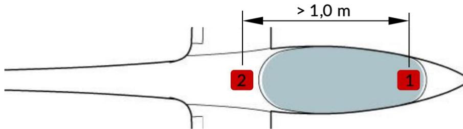
**GNSS 1 (=front) antenna** is usually mounted at the level of the instrument panel or in front of it in the nose of the aircraft.
