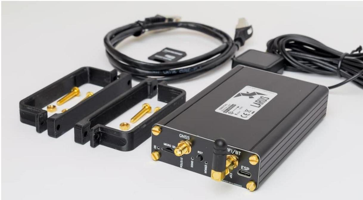
If the clamps are not ideal in your installation situation, please make sure to use only fastening material made of nonferrous materials (GFRP, aluminium, plastic, brass or stainless steel (test the latter with a magnet prior usage)).
