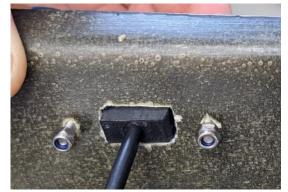
Put the same shim of the drill template onto the panel connector. Install the panel connector (please check that the white arrow on the black printed circuit board points upwards) and gently fasten the screws
