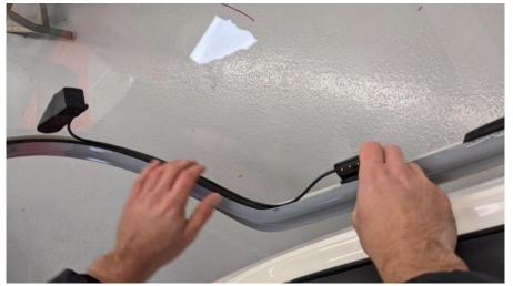
• Degrease the bonding area of the canopy and attach the side opening connector by firmly pressing it against the acrylic glass.
