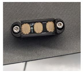
• Close the canopy carefully and check that all three POGO pins are in contact with the golden connection surfaces of the printed circuit board. For adjustment loosen the two hexagon socket screws of the canopy connector (marked with red circles), reposition, and fasten the screws again.
