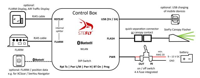
The canopy flasher is connected to the Control Box, which evaluates FLARM signals of aircraft in the surrounding area. For safety reasons (dazzling) and energy saving, the canopy flasher only emits light flashes, when the aircraft is flying. Therefore, FLARM is connected to the Control Box via a RJ45 cable.
