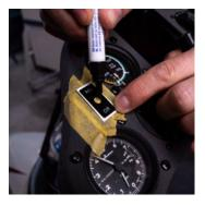
Fasten the control box in front of the instrument panel (screws and clamps / cable ties / Velcro)
