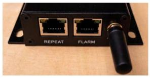
The Control Box has four status LEDs, positioned above the RJ45 connectors:
